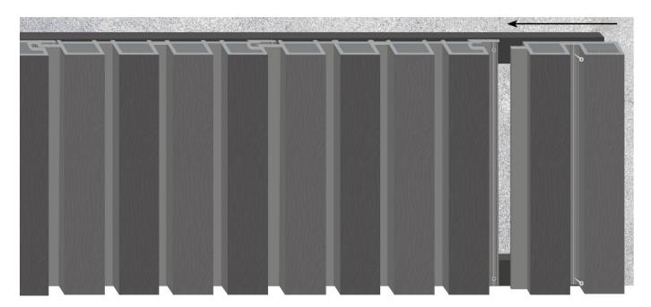
❖ Where cladding pieces meet at a butt end, a 5mm gap must be left to allow for expansion during extreme temperature.
